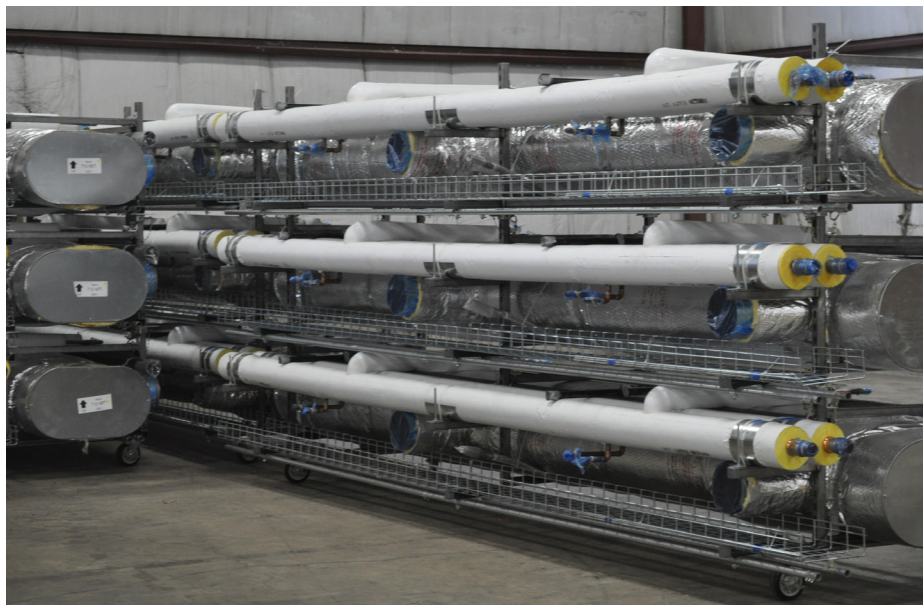
The multi-racks await transportation to the jobsite where they will be installed.
